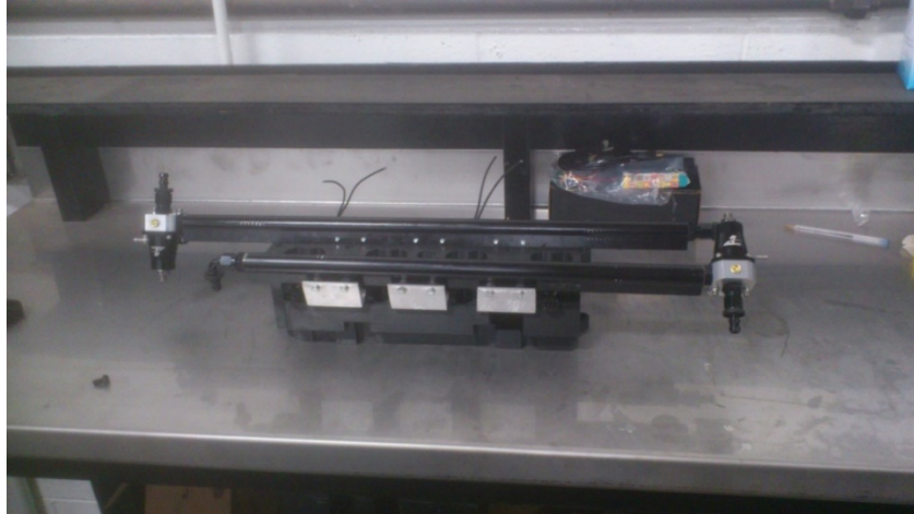
Figure A-9. PFI injector complete mounting.
