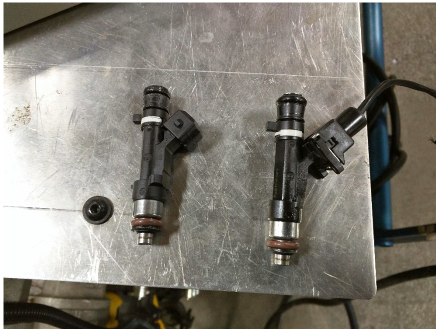
Figure A-4. EV14 EL fuel injectors with the pigtail connector
