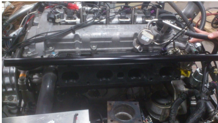
Figure A-10. PFI injector complete interface mounted on the engine.
